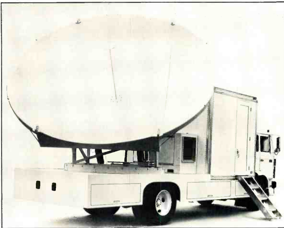
Dalsat's transportable Ku uplink
